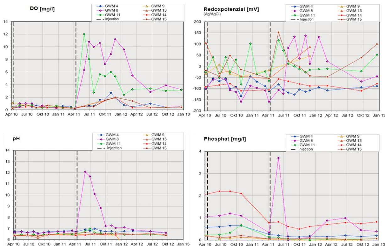
Figure 4: Effect on geochemical parameters within the treatment area.
