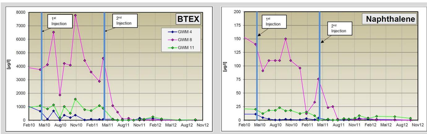
Figure 3. BTEX and Naphthalene concentrations post Injections
