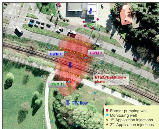
Figure 2. Phase 1 and Phase 2 Injections
